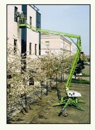
Hydraulic outriggers allow quick and easy setup and the audible alarm ensures that the operator is aware of an incorrect setup, when working in the busiest of environments.
