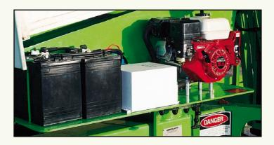
The Bi-Energy power option improves utilisation for the **140** by allowing operation in discreet and fume free environments or for extended periods where no external power source is available.
