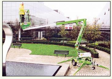
The telescopic boom provides outstanding working outreach especially at lower levels where it's needed most.
