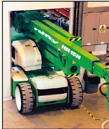
With more outreach than any other machine in its class and a base width of only 1.50m, the **HR15N** is one of the most effective and versatile self propelled platforms available.
