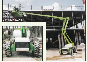
The unique suspension system shown above ensures maximum traction when travelling over uneven surfaces and the spacious 1.80m wide platform allows the operator ample room for tools and materials.
